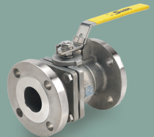
150#, 300#, 600# Flanged Ball Valves Full & Reduced Port Carbon Steel, 316 Stainless & Alloy 20 1/2" - 12"
